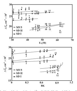
**Fig. 3** Plot of Stokes shifts (cm<sup>-1</sup>) of MV5, SD II and SD I vs.  $E_T(30)$  and BK solvent parameters: (1) cyclohexane (2) diethyl ether (3)1,4-dioxane (4) ethylacetate (5) dichloromethane (6) acetonitirle (7) *t*-butyl alcohol (8) 2-butanol (9) 2-propanol (10) ethanol (11) methanol and (12) water
