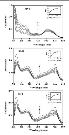
Fig. 4 Absorbance spectra of MV 5, SD II and SD I in different  $\beta$ -CD concentrations (M): (1) 0 (2) 0.001 (3) 0.002 (4) 0.004 (5) 0.006 (6) 0.008 and (7) 0.01
