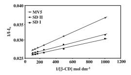
Fig. 7 Fluorescence spectra of Benesi–Hildebrand plot for the complexation of MV 5, SD II and SD I with  $\beta$ -CD (Plot of 1/I-I<sub>0</sub> vs. 1/[ $\beta$ -CD])
